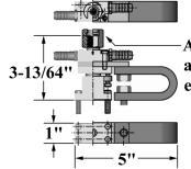
Available with tapered adapters for tapered electrodes
